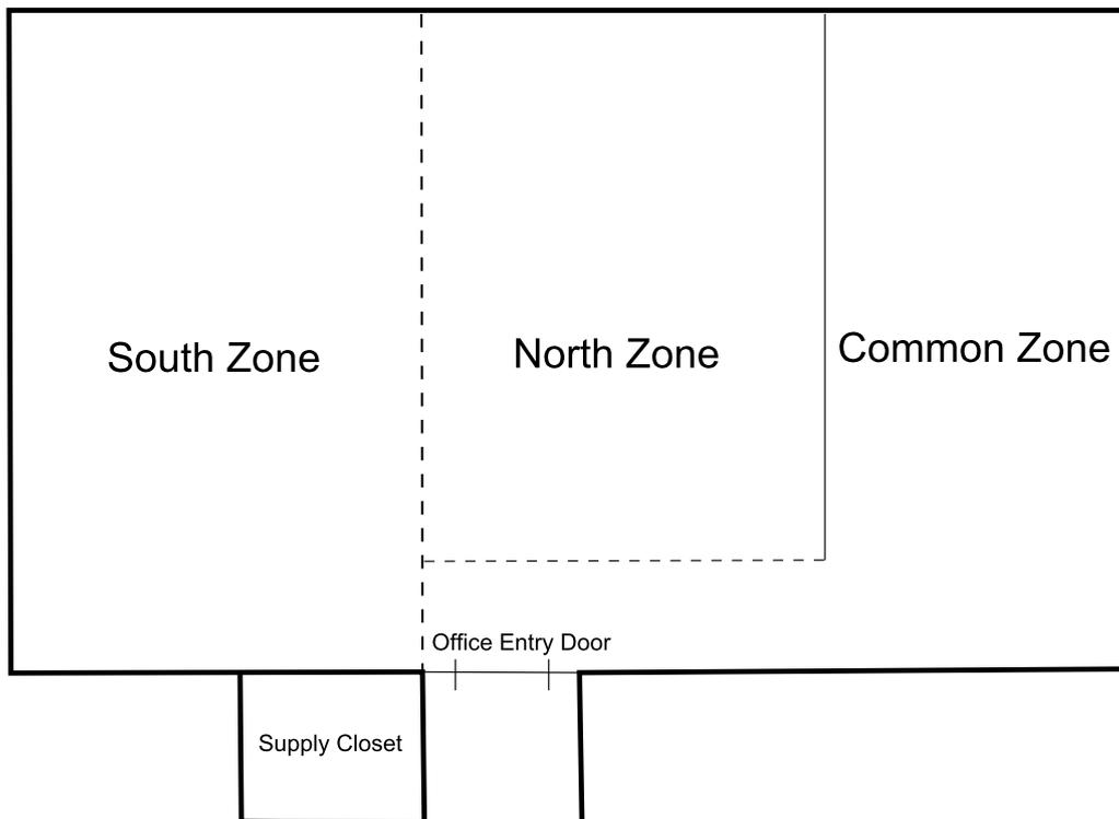
When a cleaner logs in to the keypad to disarm the Office Area, the utilities for all three zones will be activated. In addition, the lights in the supply closet will be switched on and the lock will deactivate. When the cleaner logs in to the keypad again to rearm the area, all outputs will be deactivated.
