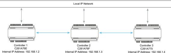
In the scenario shown above, the Protege GX server is communicating with all three remote controllers via the router. Therefore, to the server all controllers have the same external IP address: 203.97.123.169.
