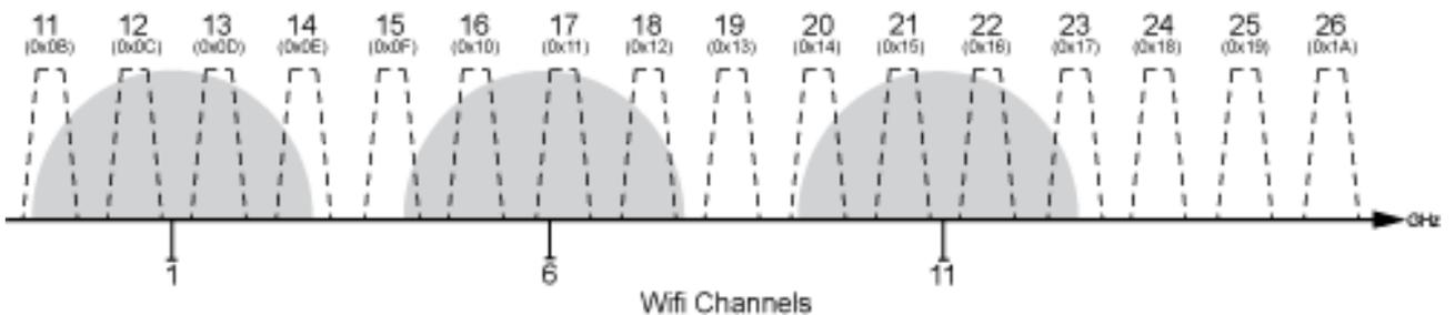
By default, AperiO hubs are configured to automatically select the radio channel that is least affected by radio interference.
