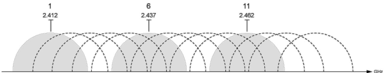
From the results of an RF site survey, you can determine which of the channels the Wi-Fi network is using. With this information, you can see which of the AperiO channels will be least affected by the Wi-Fi network. The diagram below shows that channels 11, 14, 15, 19, 20, 23, 24, 25 and 26 are the least likely to incur interference from the Wi-Fi network, so these would be the most effective channels to use for your AperiO network.
