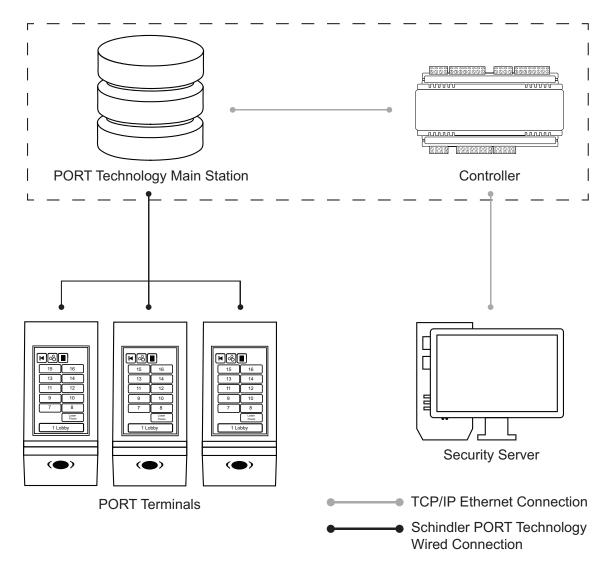
The Protege GX Schindler HLI elevator integration supports up to 128 floors.
