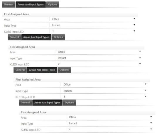
3. Here we have added the area that is associated with the keypad to all four keypad inputs, set the Input Type to Instant, and assigned a unique KLES Input LED address.
