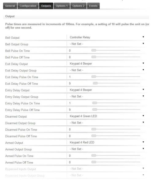
3. From here we can set the Exit Delay Output/Output Group, the Entry Delay Output/Output Group, Disarmed Output/Output Group and the Armed Output/Output Group.
