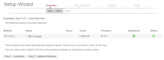
The keypad is assigned a name automatically. This can be renamed as required to provide a more meaningful name for easier identification.
