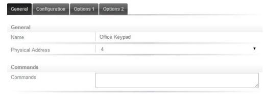
The name and physical address of the keypad can be changed from the **General** tab.
