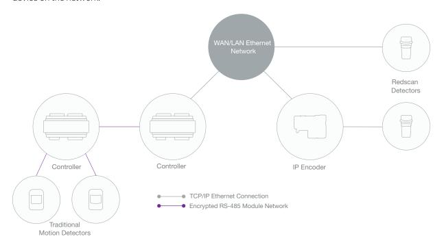
Each Redwall detector is configured as an input expander within Protege GX. The inputs and trouble inputs associated with the detectors are mapped to specific Redwall event codes, enabling you to monitor the state of the detectors. As the states change, these inputs can also generate alarms within Protege GX.
