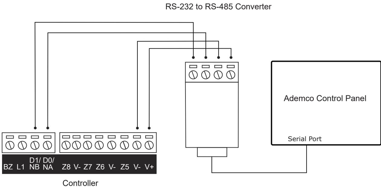
Ensure that the converter is configured to operate at 1200 Baud.
