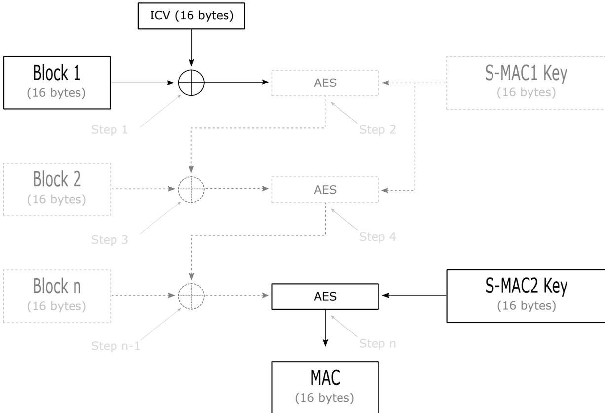
If the message size is 16 bytes (a single block) then only the S-MAC2 key will be used, as demonstrated in the diagram below.
