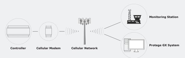
For Protege GX controllers the cellular modem also facilitates programming downloads and manual control from the Protege GX system, and event uploads to the Protege GX events database.
