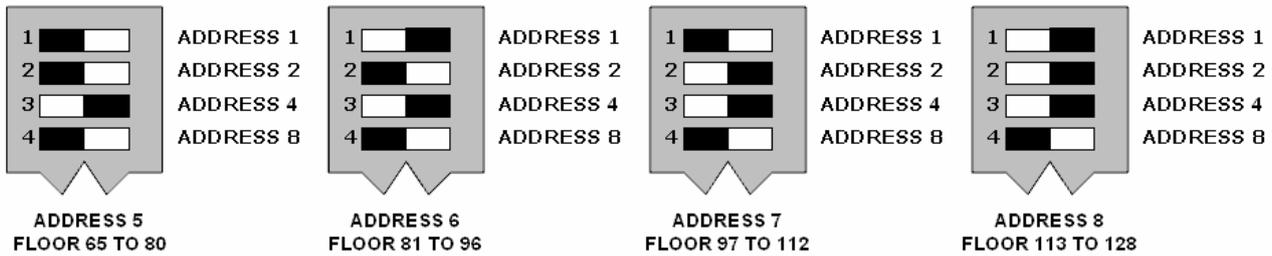
Elevator Car 1 Floor Address Configuration
