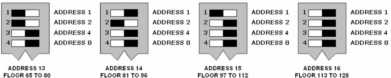
Elevator Car 2 Floor Address Configuration
