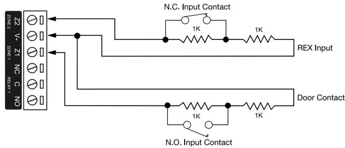
Each of these inputs can be used for either the door function that is automatically assigned or as a general purpose input. If used as general purpose inputs, make sure the inputs are not defined in the onboard reader setup.
