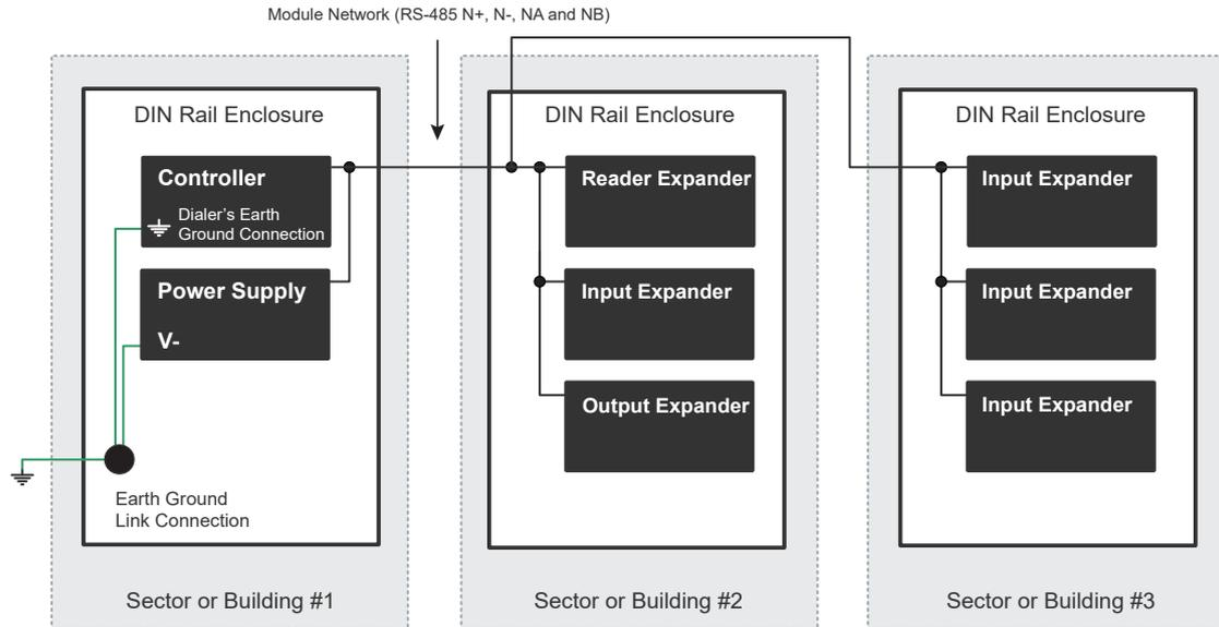
The Dialer's Earth Ground Connection applies to modem model controllers only.
