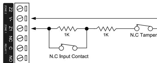
Inputs 1 and 2 can operate as either general purpose inputs or as onboard reader inputs. If used as general purpose inputs you must ensure that they are not defined in the onboard reader set up.
