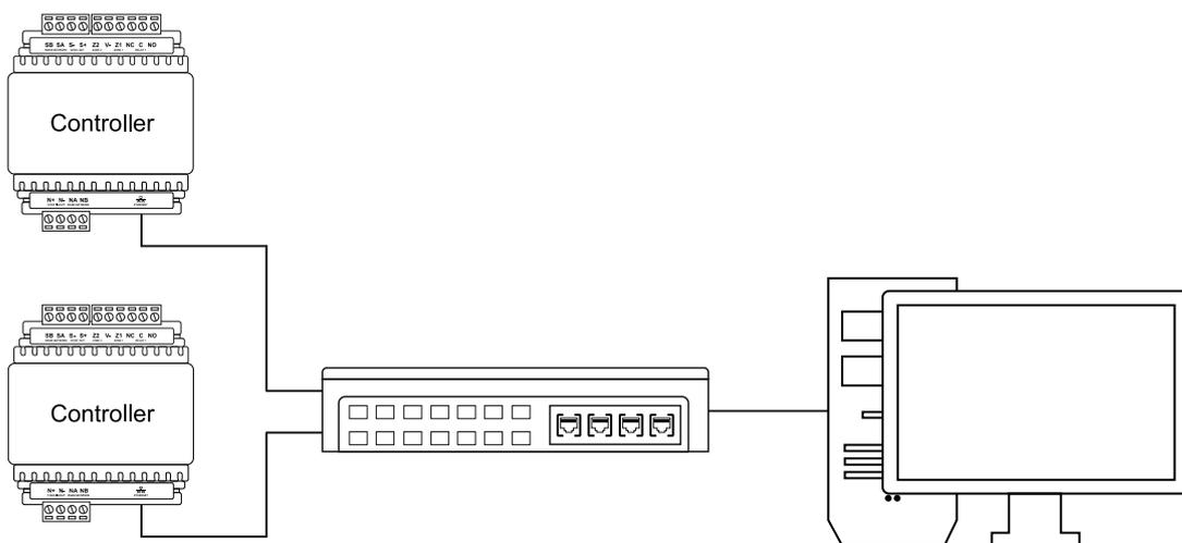
Temporary direct connections can be used for onsite programming by using a standard ethernet cable.
