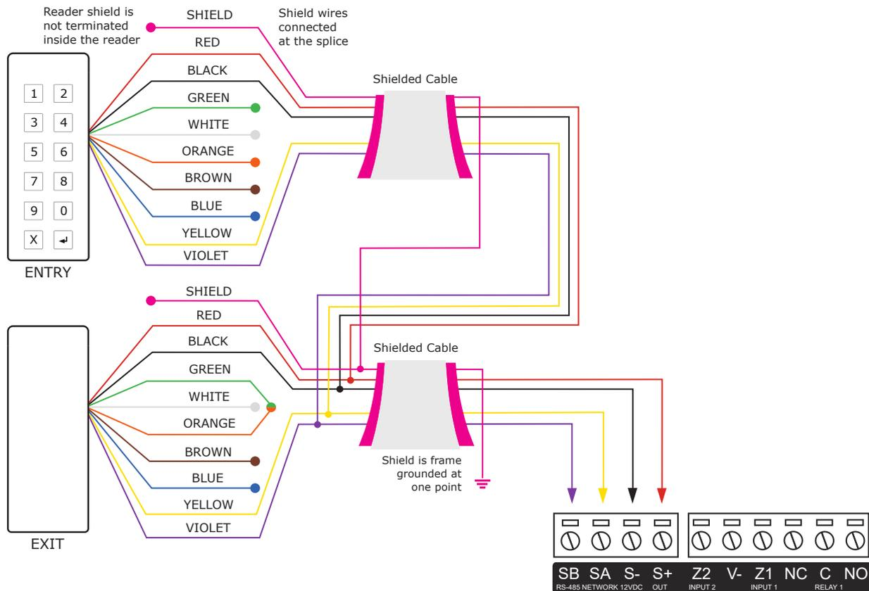
The exit reader has the **green** and **orange** wires connected together.
