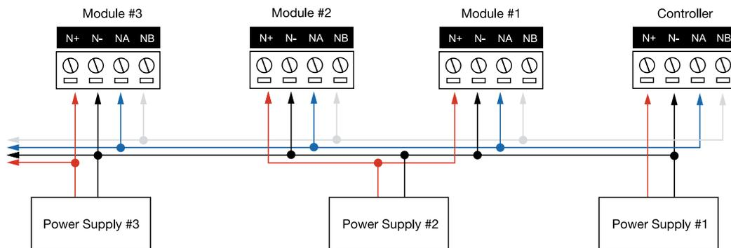
When using multiple power supplies it is important to ensure that all ground connections (V-) are connected between all power supplies and that no power connections (V+) are connected between any power supplies.
