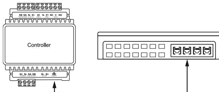
When using a PoE router as power source for the controller, the rating for the auxiliary outputs (S- S+) will be different to those when the controller is being powered by an Integrated Control Technology power supply or a 12V DC supply. Please refer to the values outlined in the Technical Specifications below for more details.
