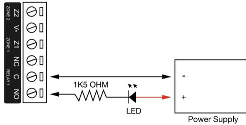
**Warning:** The relay outputs can switch to a maximum capacity of 7A. Exceeding this amount will damage the output.
