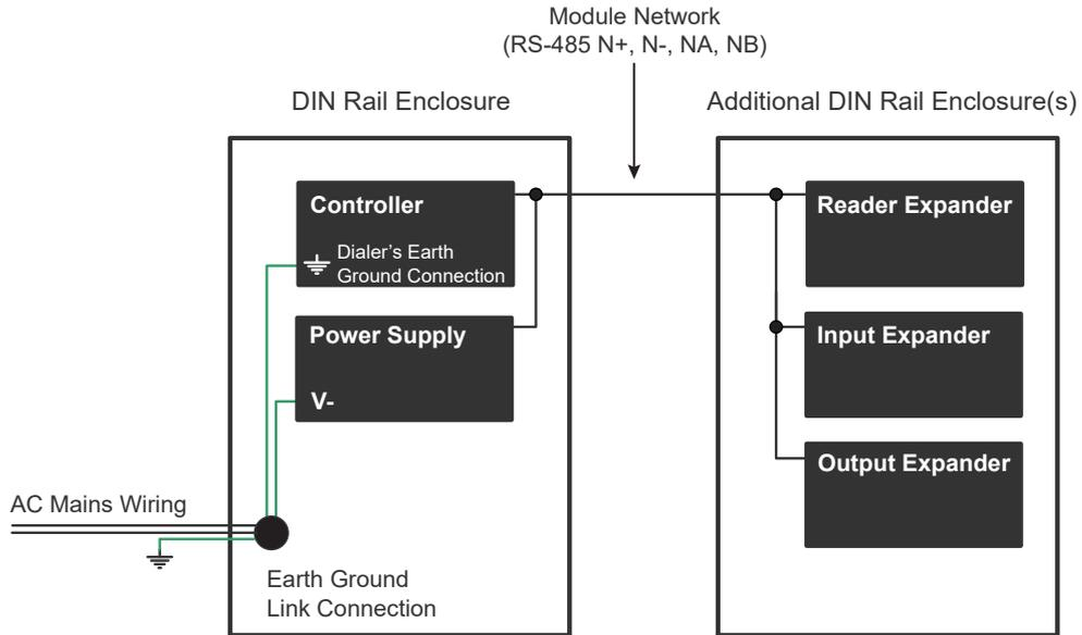
DIN Rail Ground Connections (multiple cabinets in different rooms, sectors, or buildings)
