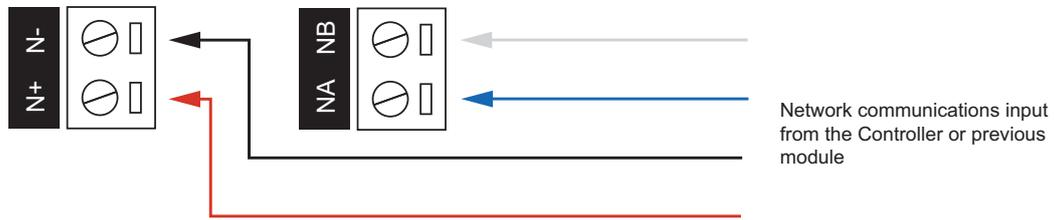
Connection of the communications and DC supply should be performed according to the diagram shown above. It is important that the N+ network communications power be 12VDC supplied from an independent battery backed power supply unit capable of supplying the required voltage to all devices on the RS-485 network.
