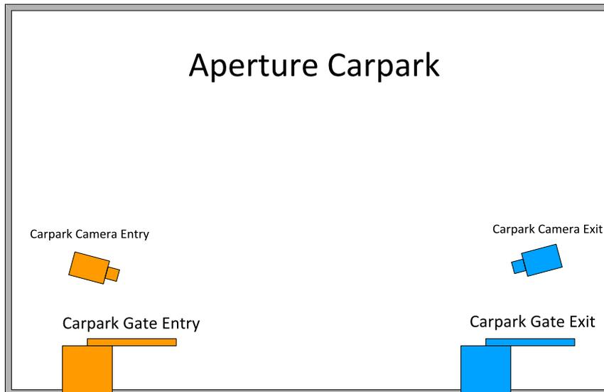
Each gate in the carpark is associated with a camera, which sends data to the controller on a specific ethernet port. Before you begin, create the door and camera records listed below.
