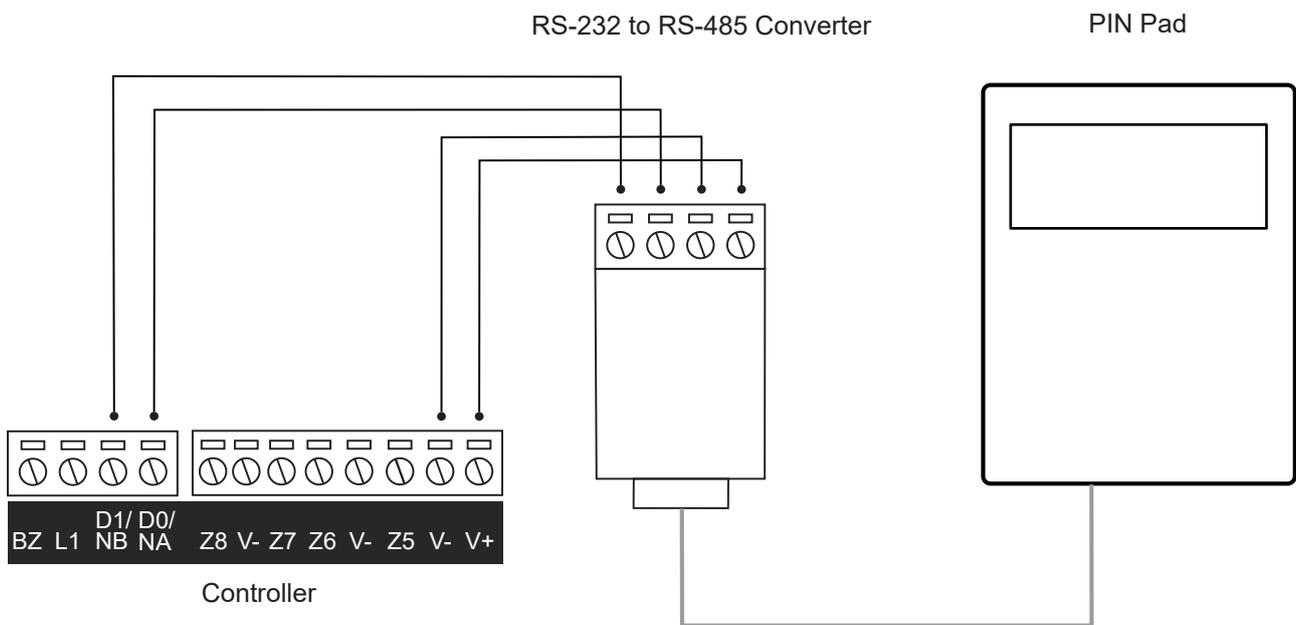
**Note:** Serial modules must be connected to the reader ports on the controller. Reader expanders can only interpret data from card readers.
