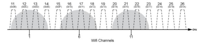
By default, Aperio hubs are configured to automatically select the radio channel that is least affected by radio interference.
