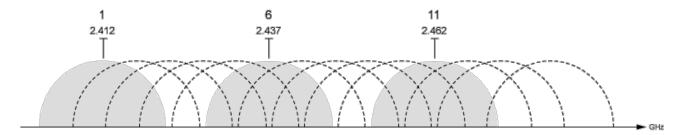
From the results of an RF site survey, you can determine which of the channels the Wi-Fi network is using. With this information, you can see which of the Aperio channels will be least affected by the Wi-Fi network. The diagram below shows that channels 11, 14, 15, 19, 20, 23, 24, 25 and 26 are the least likely to incur interference from the Wi-Fi network, so these would be the most effective channels to use for your Aperio network.
