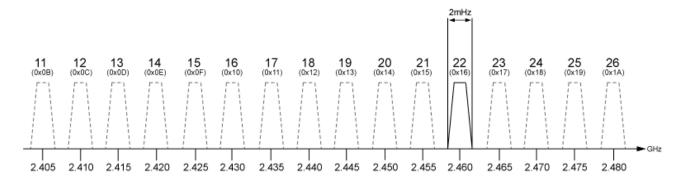
As an example, we can look at how Wi-Fi can affect the operation of Aperio when it is operating on the same 2.4GHz band. Wi-Fi generally operates on a standard of the IEEE 802.11 communication protocol divided into 14 channels, each occupying 22MHz of bandwidth from 2412MHz to 2484MHz.
