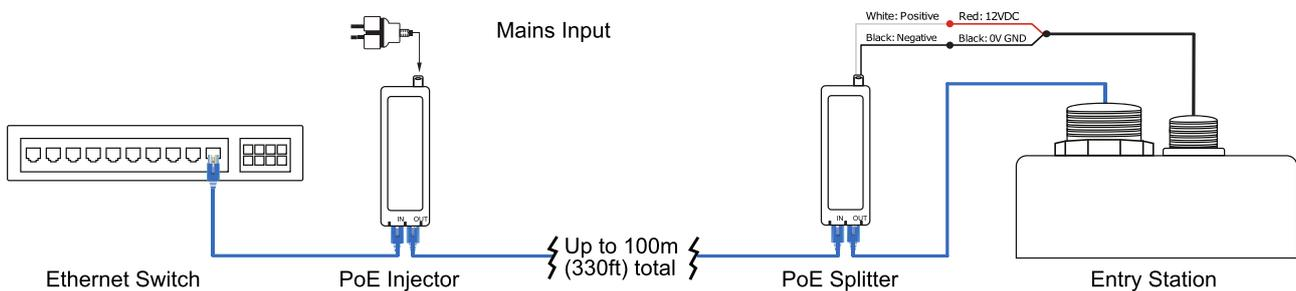
Install the PoE injector adjacent to the ethernet switch, then run the powered Cat5e or Cat6 ethernet cable to the remote location where the PoE splitter and entry station will be installed.
