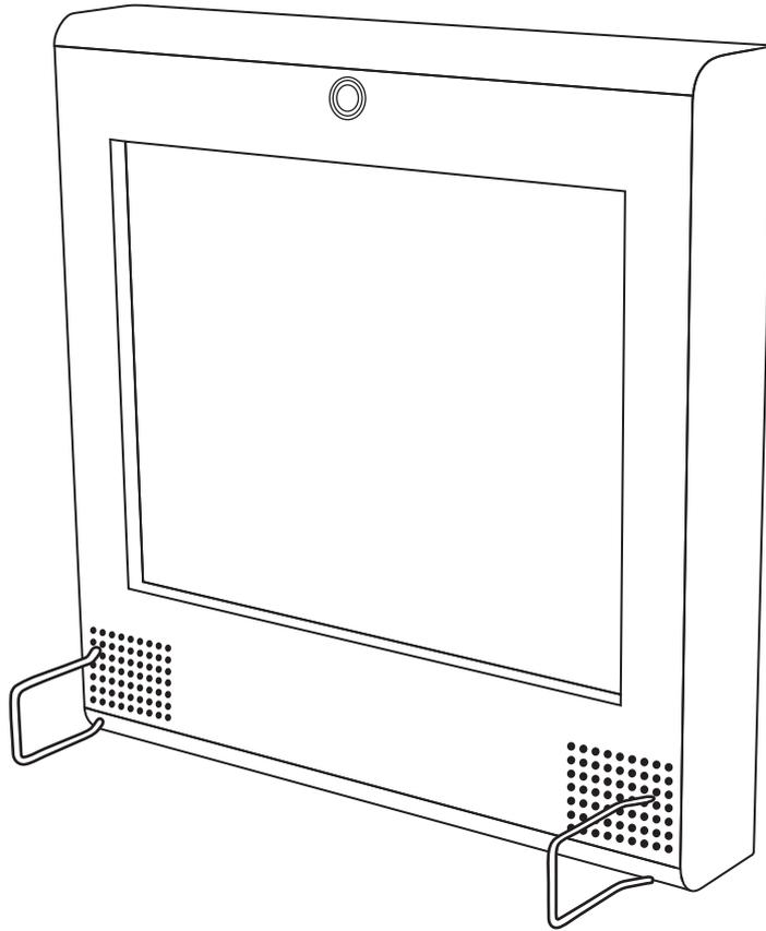
To remove the front face plate, carefully insert both of the provided tools through the outer speaker holes and push them all the way in to release the front section, then lift the cover out from the bottom.
