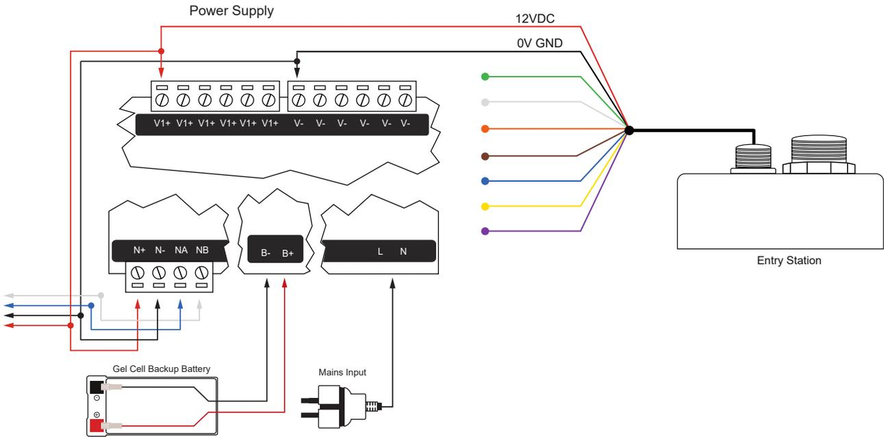
After installation, measure the input voltage at the entry station to ensure that it has a consistent supply of 12V.
