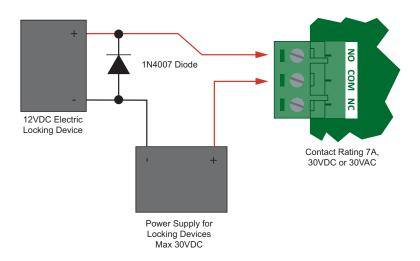
Lock Output PGM1/2 Relay Outputs
