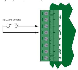
Normally Closed Zone Configuration No Resistors
