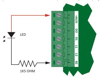
Example Open Collector Output Connection (LED)
