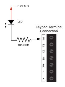
**Warning:** The open collector output can switch to a maximum capacity of 50mA. Exceeding this amount will damage the output.
