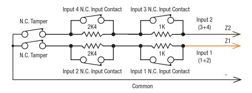
To utilize the input duplex mode configuration shown above, the **Duplex Inputs** setting must be enabled in the keypad programming (**Keypads | Options 2**).
