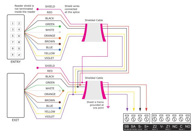
The exit reader has the **green** and **orange** wires connected together.
