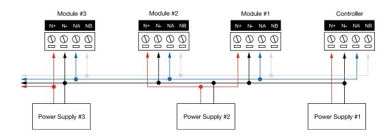
When using multiple power supplies it is important to ensure that all ground connections (V-) are connected between all power supplies and that no power connections (V+) are connected between any power supplies.
