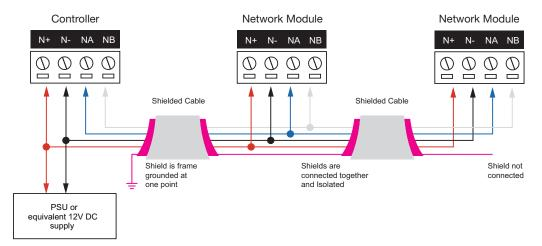
Always connect the controller's NA and NB terminals to the NA and NB terminals of the expansion devices and keypads. The N+ and N- must connect to a 12V power supply source capable of supplying the peak current drawn by all modules. If a shielded cable is used, the shield must be connected at only one end of the cable. **DO NOT** connect a shield at both ends.
