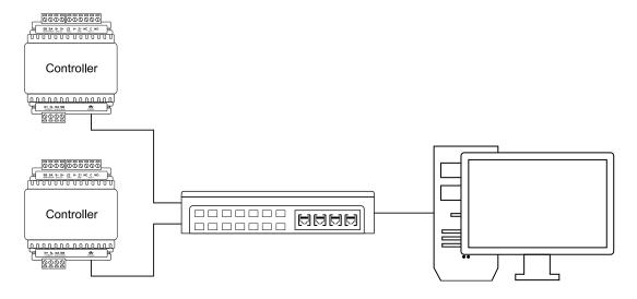
Temporary direct connections can be used for onsite programming by using a standard ethernet cable.
