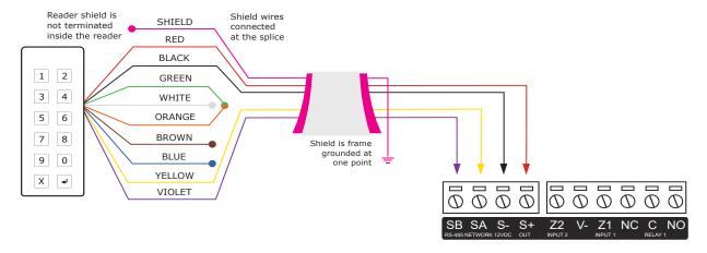
When the green and orange wires are not connected together, the reader defaults to an entry reader.
