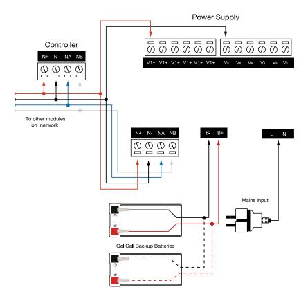
In a small installation this same power supply can be used to supply the module network as well, so long as the maximum load of the power supply is not exceeded. In larger installations, the power supply may need to be split to allow for load sharing between several supplies.
