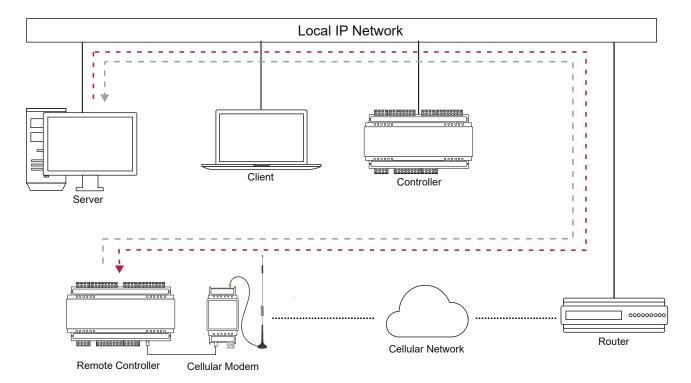
Protege GX controllers can also use the Protege DIN Rail Cellular Modem to communicate with the server via the 4G cellular network. This allows you to connect controllers to the Protege GX system even when they are located outside of wired networks.
