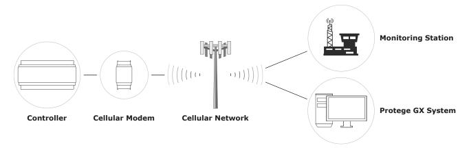
For Protege GX controllers this device can provide wireless IP alarm transmission capability, and on supported networks can also facilitate programming downloads and manual control from the Protege GX system, and event uploads to the Protege GX events database.
