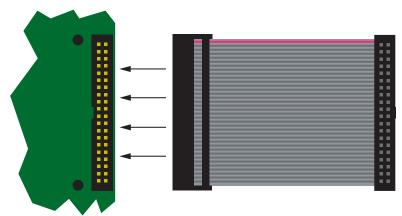
Expansion Connector and Mounting Hole Location
