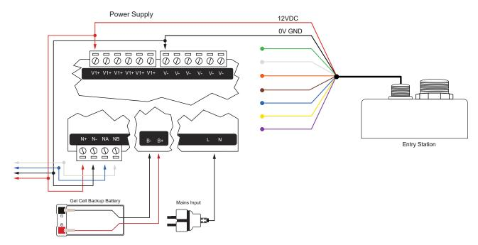
After installation, measure the input voltage at the entry station to ensure that it has a minimum supply of 10V.
